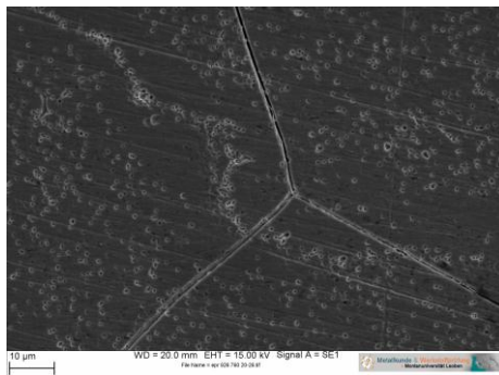
c) 760_20 after EPR-test: continuous intergranular corrosion
