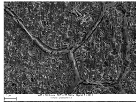
d) 900_120 after EPR-test: intergranular and uniform attack
